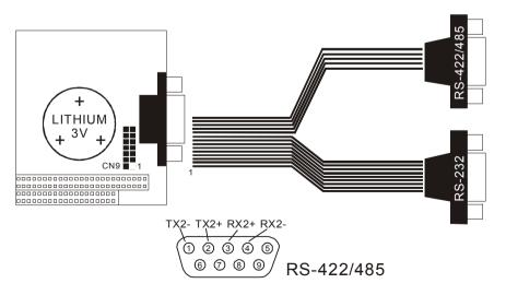
**Note** : TX2+,TX2- and RX2+,RX2- are for transmitting and receiving, respectively, in the RS-422 connection. While in RS-485 connection, TX2+,RX2+ and TX2-,RX2- must be twisted each. Anyhow, you can only choose to use **RS-232** or **RS-422/485**.
