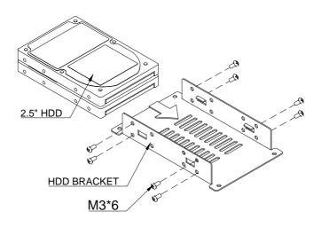
Step2. Place the whole modules into the cabinet, and fasten them with screws shown in the diagram.
