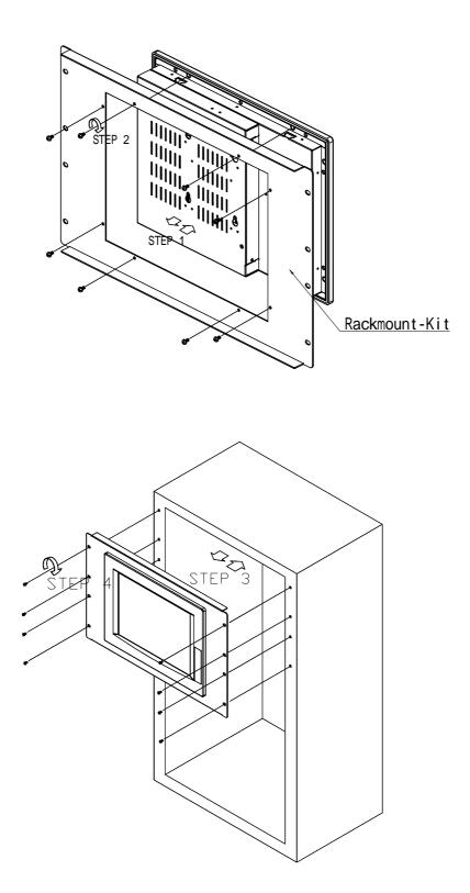
Appendix A Exploded Diagram of PPC-5150 With Aluminum Front Panel
