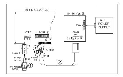
Connect the ATX power button switch to the pin 17 (power button) and pin 19 (+5VSB) of CN18 on the board. And connect the power cable from CN4 of backplane to CN16 of CPU card.
