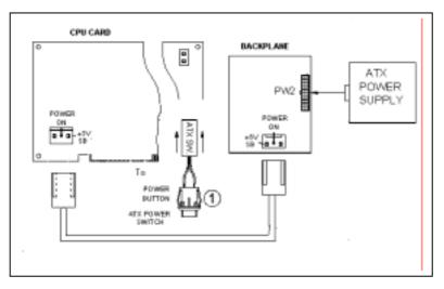
Connect the ATX power button switch to the CN5 (power button). And connect the power cable from backplane to CN20 of CPU card.
